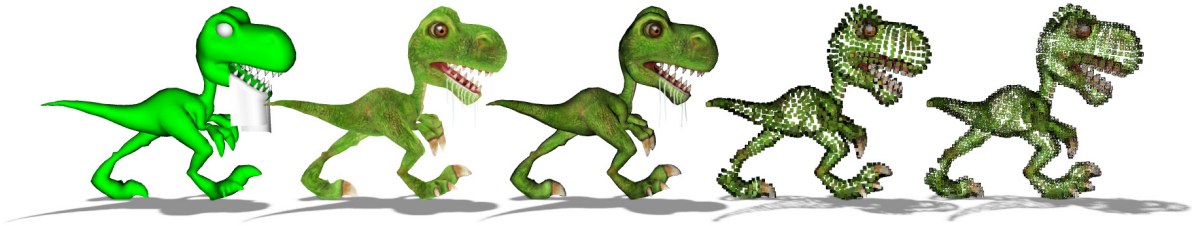
Figure 1: Example built with composed shader modules (from left to right): transformation and per-pixel lighting, transformation and texturing, transformation/normal mapping/texturing and lighting, transformation/normal mapping/texturing/point sprite generation and lighting, transformation/normal mapping/texturing/point sprites/thick line generation and lighting.
